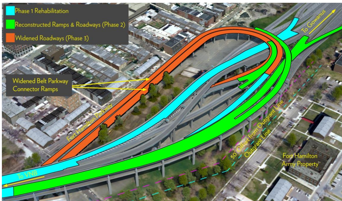
Figure 3-2: Brooklyn Upper Level Approach Ramps – Rehabilitation Phases
