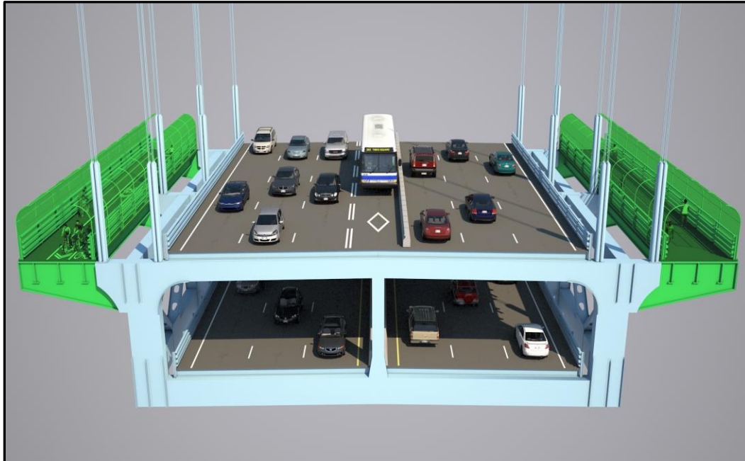
Figure 5-7: Upper Level Outboard Shared-Use Path – Cross-Section
